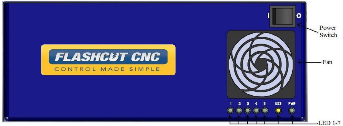
The front panel of the CNC controller has the power switch, the fan and 7 LED's with the following functions:
