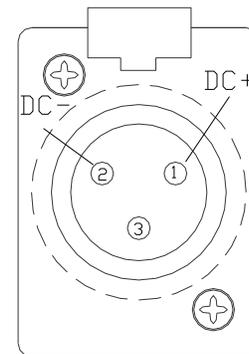
Connectors on Cables are DB15 Male and a Male Audio Connector (Neutrik NC3MX or equivalent).
