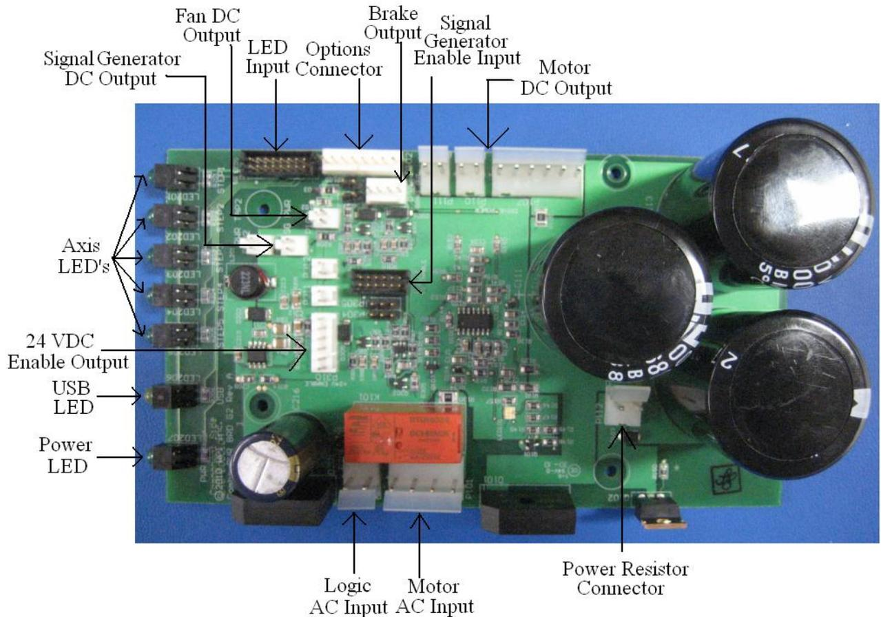
The function of the Power Board is to supply DC voltage to the drive modules as well as to the cooling fan and logic signals to the Signal Generator. The power enters the board in the form AC voltage from a transformer; the AC voltage is then converted to DC voltage. The Power Board also contains the indication LED's:
