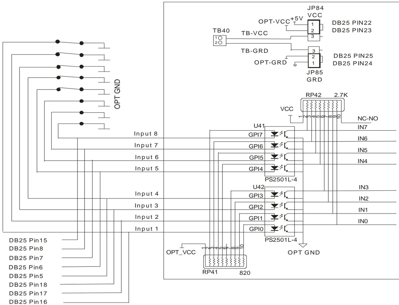
The above schematic shows a typical connection of 5 normally closed switches. These switches are connected between input lines 1-5 and ground. Lines 6-8 are connected directly to ground with jumper wires. All external connections shown are made through the Input connector on the back of the Signal Generator. This resistor pack (RP41) is socketed so that you can change the value if needed for your application.
